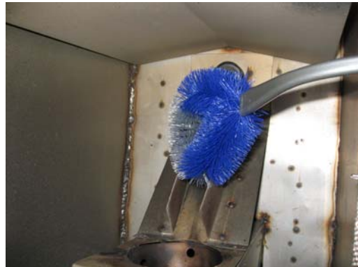
Figure 6 – Pellet Slide Cleaning
