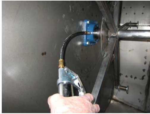
Figure 3 - Greasing rotisserie bearings
