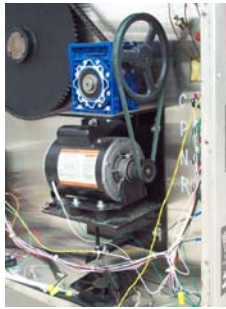
Figure 4 - Rotisserie drive chain and tension adjustment
